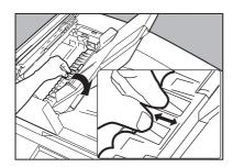
Open the Exit Guide while holding the green labeled tab.
