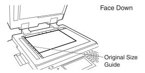
Place a book or an original Face Down on the Platen Glass, aligning it with the arrow mark on the original size guides.
