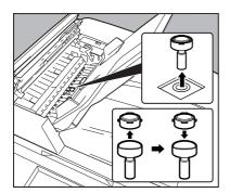
1. Remove by pulling the Stamp Assembly upward.
