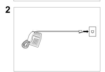
Plug a different regular telephone into the same telephone jack.
