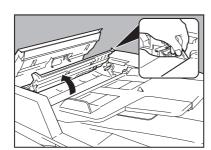
Open the Inner Cover with holding the green-labeled tab.
